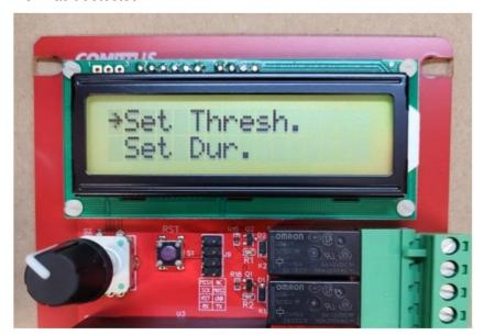
Select "Set Threshold" - alarm on speed
