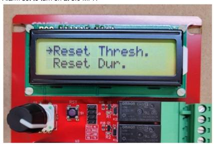
Select "Reset Threshold" - alarm off speed
