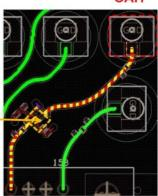
Trace Length: 677.21mil Trace Width: 12.5mil PCB thickness: 1.6mm Dielectric constant: 4 (FR-4)
