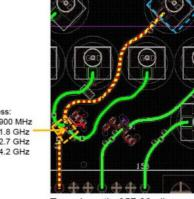
Trace Length: 957.29mil Trace Width: 12.5mil PCB thickness: 1.6mm Dielectric constant: 4 (FR-4) Trace copper foil: 1oz
