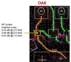
Trace Length: 627.04mil Trace Width: 12.5mil PCB thickness: 1.6mm Dielectric constant: 4 (FR-4) Trace copper foil: 1oz
