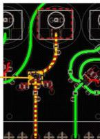
Trace Length: 473.64mil Trace Width: 12.5mil PCB thickness: 1.6mm Dielectric constant: 4 (FR-4) Trace copper foil: 1oz
