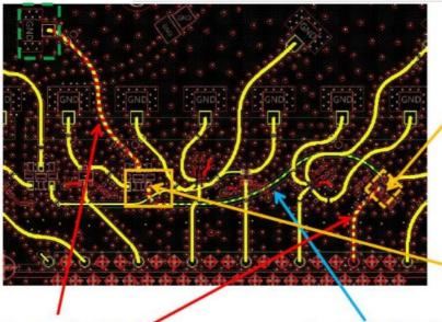
Trace Length: 857.28mil Trace Width: 12.5mil PCB thickness: 1.6mm Dielectric constant: 4 (FR-4) Trace copper foil: 1oz
