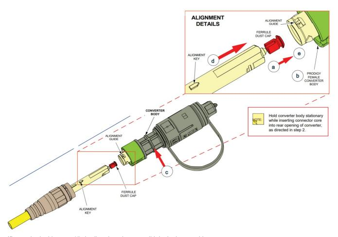
(f) turn the locking nut  $45^{\circ}$  in direction shown until it locks into position.
