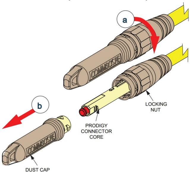
2. Install the female converter as follows: (a) remove the red ferrule dust cap from the Prodigy connector, (b) locate Prodigy female converter, (c) hold onto converter body to keep it from turning, (d) Roughly align the alignment key on Prodigy connector core with alignment guide in converter body; (e) insert the connector core all the way in.
