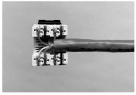
After terminating. Slide the strain relief onto the modular jack until the latches of the strain relief engage of the modular jack as shown in Figure 5.
