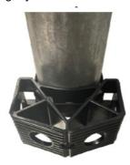
3. Configuration showing adapter securely attached to round member. Maximum hanger loading is twelve 4-17 mm hangers or eight 26-42 mm hangers.
