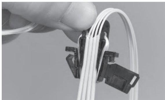
12. Installation of third and fourth pigtail at the opposite side of the KTU.
