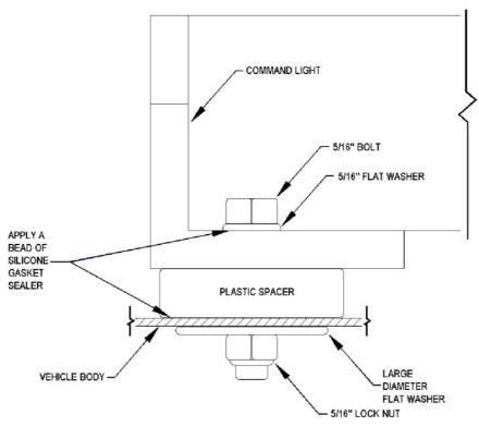
Drill 21/64" holes in the mounting surface using the end casting holes as a template.
