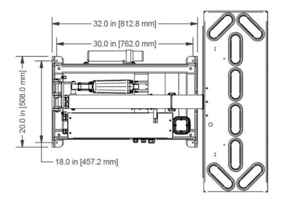
Four mounting bolts are required. Additional holes may be drilled in the frame ends if necessary to clear obstructions.
