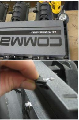
Drill out the four holes using a 5/16 drill bit, leaving the dust cover in place. Remove the dust cover and attach the four clip-on nuts to the side panel.
