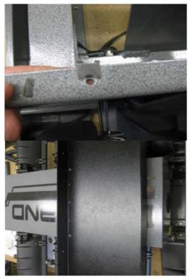
Align the clips with the drilled holes. Place the dustcover back in place with all screws except for the top four. With
