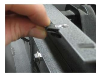
Drill out the four holes using a 5/16 drill bit, leaving the dust cover in place. Remove the dust cover and attach the four clip-on nuts to the side panel.
