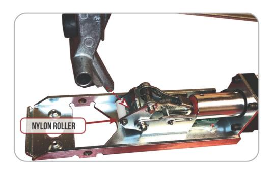
5. Once the point is in the opening, depress the push pad until the holes on the activating bracket & motor mount line up. Re-install factory pin.
