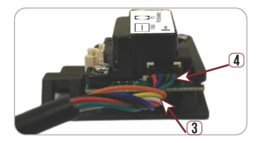
10. Using double sided tape, secure MM5 to inside of the back of exit device housing. Connect Molex Pigtail. Add Mounting Pad & cable tie to secure cable wires.
