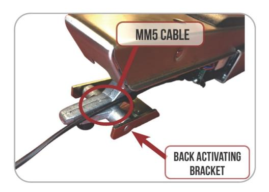
9. Plug-in cable's (4) Pin TOP port & (3) Pin BOTTOM port into MM5 ports.
