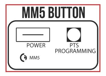
Step 1 – To enter PTS mode: Depress MM5 button & apply power. The device will emit 1 SHORT beep. The device is now in PTS mode.
