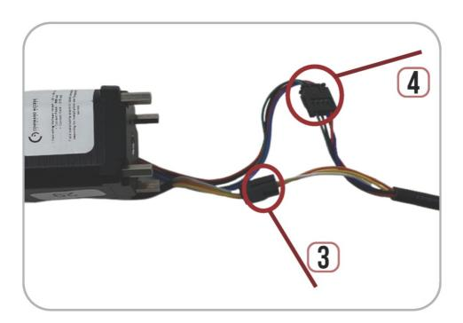
7. Slide Push Pad & Motor Kit back into housing. Be cautious of MM5 cable wires.
