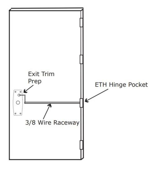
Run the wires from the ETH hinge through the 3/8" raceway starting at the ETH hinge & exiting into the pocket
