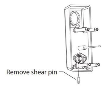
• Rotate the lever to the desired position. Re-install shear pin
