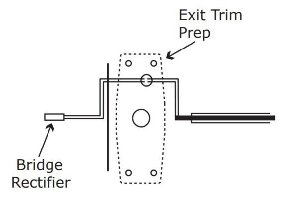
Connect the Bridge Rectifier to the plug exiting the Electric Exit Trim
