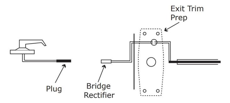
Carefully slip the connected Electric Exit Trim into the pocket paying close attention not to pinch any wires.
