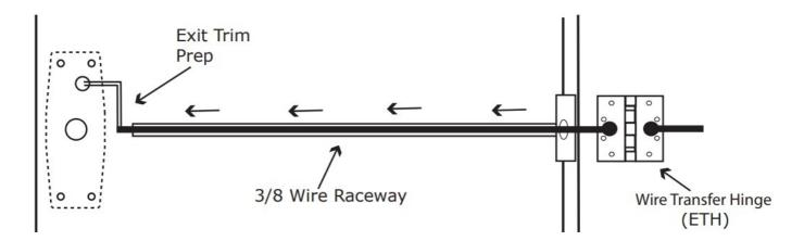
: Screw the ETH hinge to the door. At this time DO NOT connect the hinge wires on the jamb side to the wires coming from the power supply.
