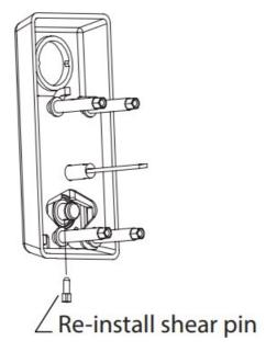
• Re-install lever cam with the correct letter visiable. R=RHR & L=LHR
