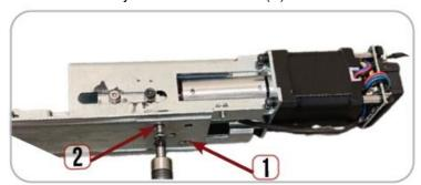
5. Slide the (B) Connecting Bracket over the Dogging post at the end of the push pad. Next, move Attaching Arms
