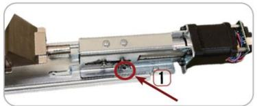
4. Turn full assembly to the side & install (E) Screws from underneath to secure motor kit to Base Rail.
