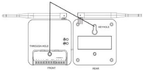
CAUTION: DO NOT OVERTIGHTEN LOWER MOUNTING SCREW, MAY DAMAGE SMART HUB.
