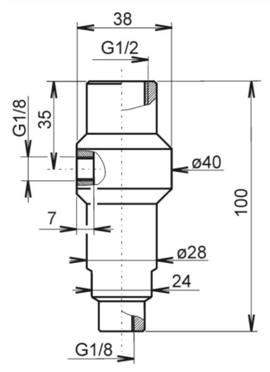
Material of flow chamber: stainless steel (DIN 1.4301)
