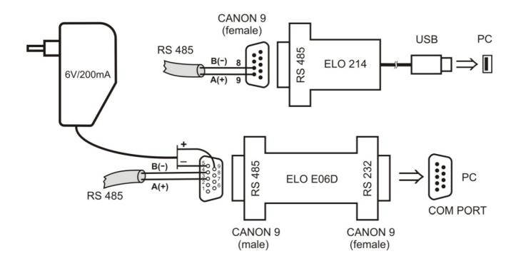
The **ELO E214** converter is an optional accessory for connection of transmitter with RS485 interface to the PC via USB port. Link RS485 is connected across pin 9 A(+) and pin 8 B(-). The pull up, pull down and termination resistors are part of the transmitter. These internal resistors can be connected to the bus by connecting the
