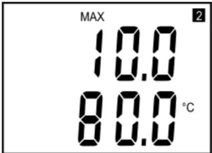
After next press of the button value for upper point appears, here 10 V corresponds to ambient temperature +80 °C. Press button again to end info mode and display actual measured values.
