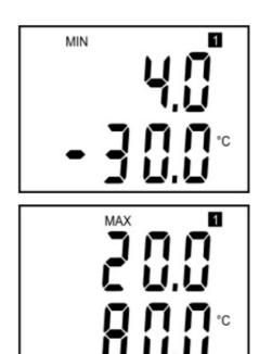
Notice: during info mode no measurement and no output current generation proceed. The transmitter stays at info mode 15 s and then automatically goes back to measuring cycle.
