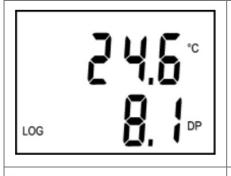
Every 5 s display is automatically switched to displaying of other measured or calculated quantity. Logger now displays ambient temperatur e and dew point temperature (LCD line marked by symbol DP).
