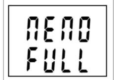
If measured value is out of the measurable or displayable range numeric r eading is replaced by hyphens. If memory is totally full filled in non-cyclic I ogging mode, logger is switched OFF and message MEMO FULL appears on the LCD. It appears also if logger is operated with switched OFF displa y.
