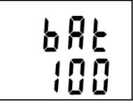
Consequently reading of estimated remaining battery capacity for approximately 2 s is displayed (values 0 to 100%). It is valid if logger is operated at temperature from -5 to +35°C. If logger is operated often outside of the above temperature range battery life can be reduced to 75%, i.e. if display ed remaining battery capacity drops below 25%, it is recommended to replace the battery.
