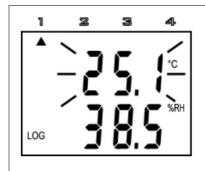
Active alarm is indicated (if display is ON) by blinking of the value of prope r quantity on the display and arrow symbol appears at the LCD upper side at the same time. Arrow 1 indicates active alarm for ambient temperature, arrow 2 relative humidity and arrow 4 dew point temperature. Notice: if log ger is operated at low temperature (below approximately -5 °C), alarm indication by blinking can be indistinct. Indication by arrows works correctly.
