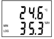
Switched ON logger permanently (with 10 s interval) updates memory of minimum and maximum values of each measured (or calculated) quantity. If displaying of MIN/MAX values is selected, minimum measured values ar e displayed step by step (indicated by symbol MIN) and then similarly maximum measured values of all quantities (indicated by symbol MAX). The entire cycle is repeated periodically, i.e. reading of actual measured values follows.
