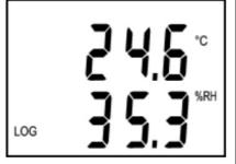
If display is switched ON, actual reading of measured values is displaye d – ambient temperature (°C) on the LCD upper line, relative humidity (%R H) on the LCD lower line. Symbol LOG indicates data logging in progress – if it blinks, data memory is filled up to more than 90%.
