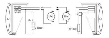
maximum load current of voltage output is 0.5 mA
