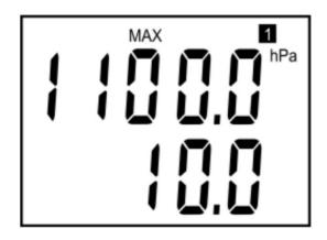
**Notice:** during info mode no measurement and no output current generation proceed. The device stays at info mode 15 s and then automatically goes back to measuring cycle.
