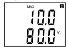
**Notice:** during info mode no measurement and no output voltage generation proceed. The transmitter stays at info mode 15 s, and then automatically goes back to measuring cycle.
