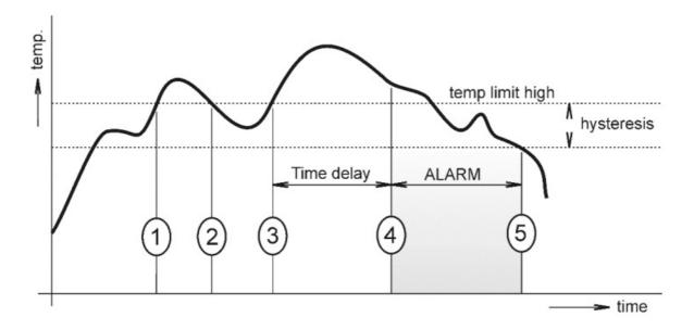
In Point 1 the temperature exceeded the limit. From this time, the time-delay is counting.
