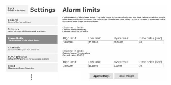
• Example of setting the limit to the upper alarm limit:
