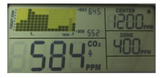
The device constantly displays current ambient CO2, set center value and set zone value.
