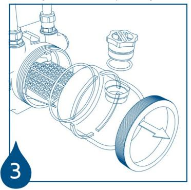
4. Refit red filler plug and replace front cover. Hang spanner on hook.
