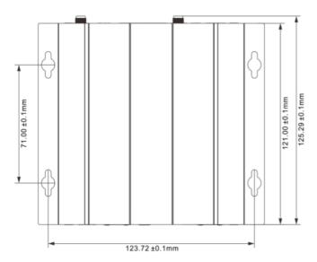
Installation method fix the device to the screen or the wall with 4 bolts or nuts of which the diameter is 3mm.
