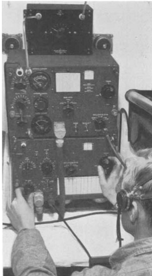
Model TOS transmitting-receiving equipment set up for operation The antenna loading coil is mounted on top of the transmitter.
