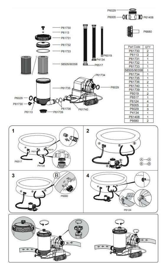
**NOTE:** You must clean the filter cartridge every day and open the top valve let the air out then close it before using the pump, otherwise the pump may not work.
