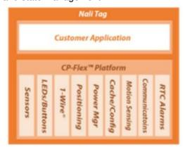
The platform efficiently manages wake and sleep states, communications, and other functions notifying the script when changes occur. Using the script capabilities, developers have full access to the device's functions without having to deal with complex embedded firmware.
