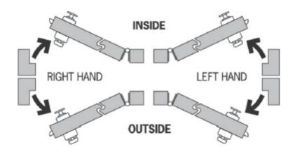
Viewed from the outside, a door is right-handed if the hinges are on the right, and left-handed if the hinges are on the left.
