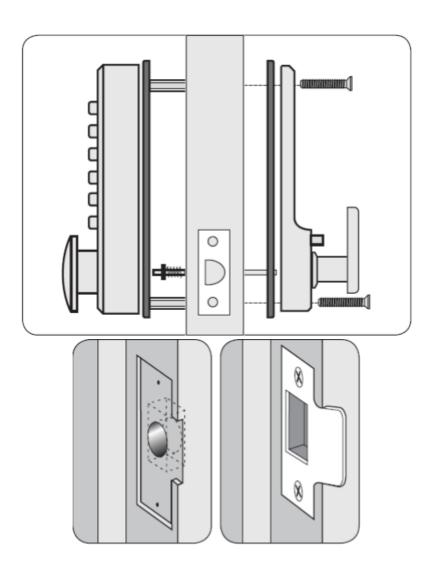
**NB** The plunger beside the latch bolt deadlocks the latch bolt and protects it against manipulation. IT MUST NOT enter the strike plate aperture when the door is closed.
