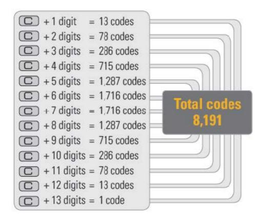
Generally codes are set in the range of 4 to 7 digits, and the total number of codes in this range is 5434. The lock is factory set with a randomly selected 6 digit code starting with the '
