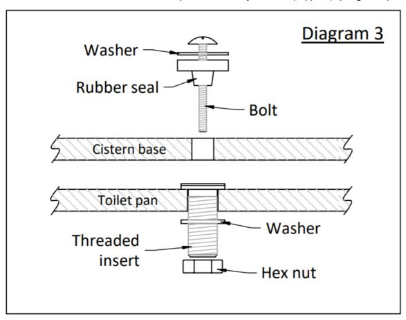
• Secure the cistern to toilet pan by screwing the cistern fixing bolts and washers to the threaded insert. Screw
