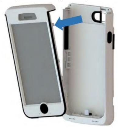
Before inserting the iPhone, thoroughly clean the iPhone screen and both sides of the glass screen protector. Screen responsiveness will be hindered if the screens are dirty. Insert the iPhone into the top plate; it will click into place.
