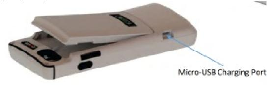
The battery fuel gauge LEDs will light up, indicating the battery's state of charge. The table below presents the charge definition per LED. The LEDs will turn off after approximately 15 minutes once the battery is fully charged.
