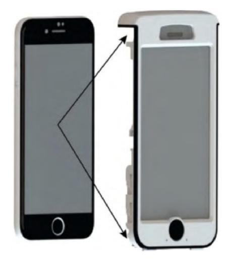
Replace the top plate into the bottom carriage directly above the lightning connector, similar to the removal process; the top plate will be inserted approximately 5 millimeters from the edge of the bottom carriage. Push down on the top plate to secure the iPhone onto the lightning connector and seal the case.
