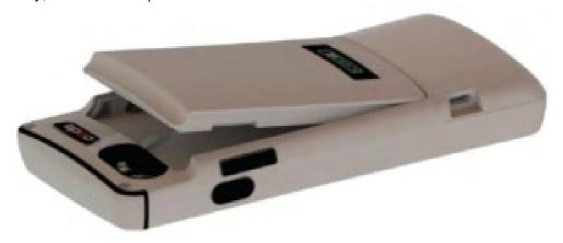
The fuel gauge LEDs will light up, indicating the battery's state of charge. If the LEDs do not light up, fully charge the battery before using.
