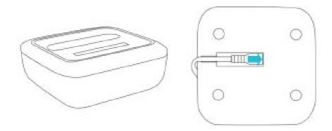
Load Battery or Case as shown. It is recommended to fully charge each new battery before the first use even though a new battery may have residual power upon receiving.
