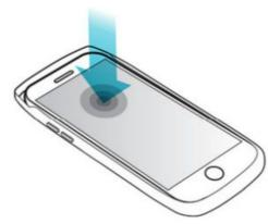
5. Align cover with side rails and slide the cover down.
