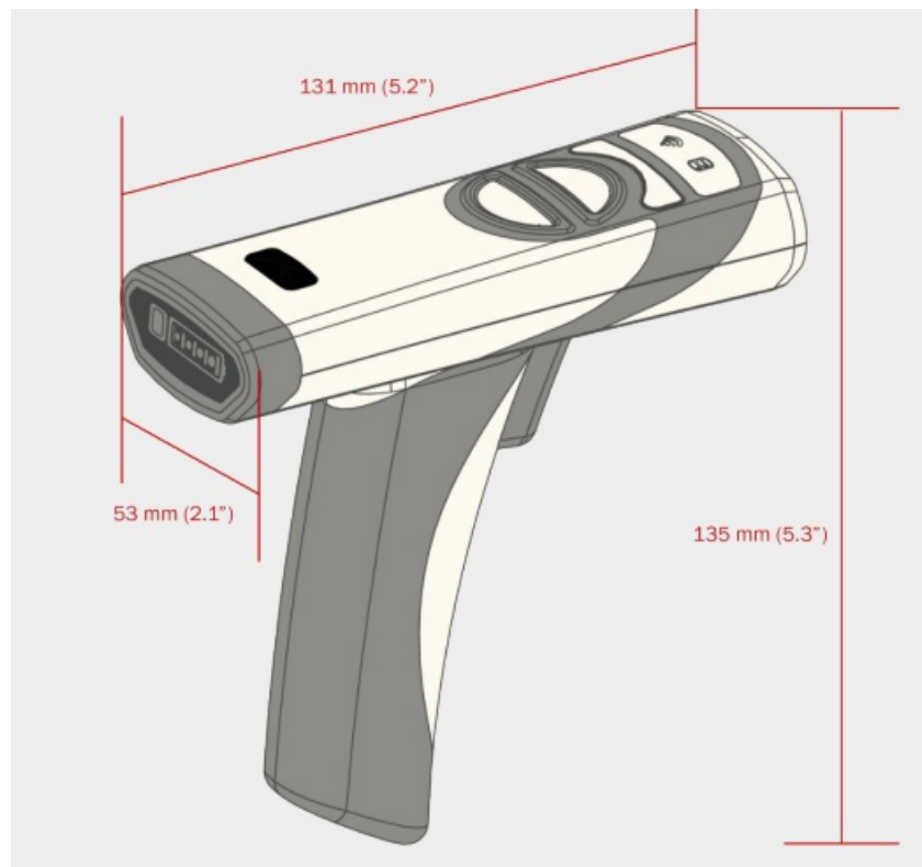
Figure 16: CR2702 Reader Dimensions
