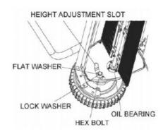
**NOTE:** To remove wheel, use a screwdriver to pop off hub cap, remove the lock nut and washer.
