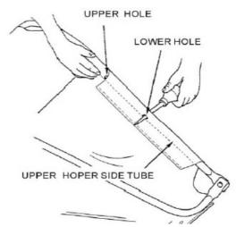
• On each side, mount a bag arm tube onto the upper hopper side tube, then insert a F plastic spacer Ø8
