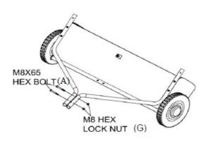
• STEP 4: Mount Hitch Assembly to Hitch Tubes
