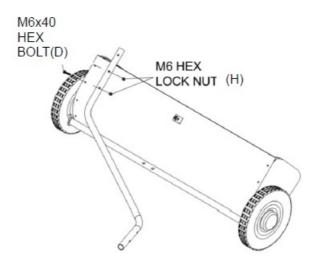
• STEP 3: Secure Hitch Tubes Together
