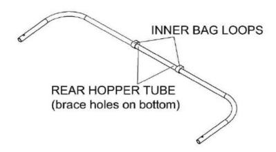
Pass the upper hopper side tubes through the stitched sleeves on either side of the nylon fabric. On each side, insert the upper hopper side tube into the rear hopper tube, oriented downwards, and fasten plastic plugs (Z).
