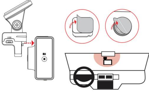
To install the Adhesive Windshield Mount, slide the dashcam onto the mount. Remove protective film from the camera lens and display. Find the spot on your windshield where you would like to mount the camera and confirm the placement. Reminder, this is an adhesive mount, so it is important to mount correctly the first time. Next, peel the plastic film of the 3M adhesive and press the mount FIRMLY onto the windshield.
