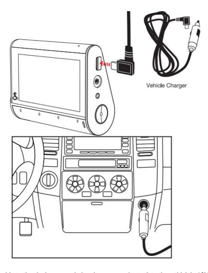
Connect the USB-C cable to the dash cam and plug the power adapter into the vehicle's 12V port
