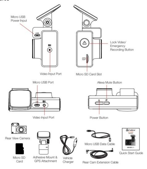
1. Attach the GPS mount to the main camera and remove the protective film from the mount and camera lens
