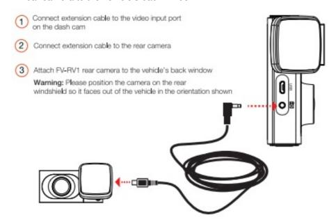
Warning: Please position the camera on the rear windshield so it faces out of the vehicle in the orientation shown
