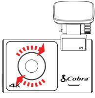
Rotate front bezel to reduce glare
