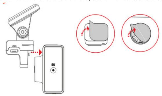
2. Connect the Micro USB cable into the GPS mount plus the power adapter into your vehicle's 12V port.
