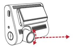
Rotate front camera lens so that it is parallel with the road.
