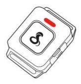
**NOTE:** Fully charge your All Road PTT Button before use. When the LED indicator is blinking red, the battery level is low and it is time to charge the PTT button.
