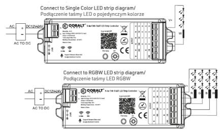
The controller input voltage must be in accordance with the required voltage of LED Strips. String Length: 9-10mm
