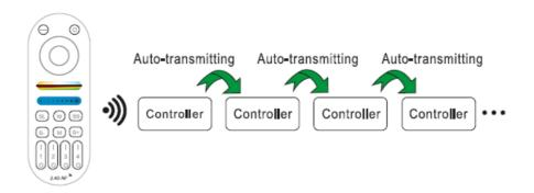
One strip controller can transmit the signals from the remote control to another controller within 30m, as long as there is a strip controller within 30m, the remote control distance can be limitless
