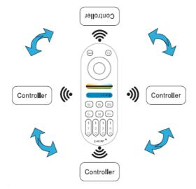
Different controllers can work synchronously when they are started at different times, controlled by the same remote, under the same dynamic mode, and with the same speed.
