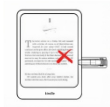
Wrong: Not clamped in the reading area
