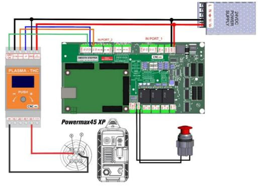
**Note** This wiring is just to illustrate a sample product application. Specific wiring may vary from system to system. It is the users responsibility to implement it correctly.
