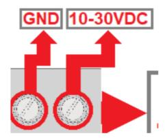
**WARNING:** Check the polarity and voltage of the external power source and connect the 10VDC to 30VDC and GND. Overvoltage or reverse-polarity power applied to these terminals can cause damage to the board, and/or the power source.
