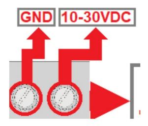
**WARNING:** Check the polarity and voltage of the external power source and connect the 10VDC to 30VDC and GND. Overvoltage or reverse-polarity power applied to these terminals can cause damage to the board, and/or the power source.
