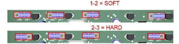
Use Hardware Enable to keep the driver enabled all the time.
