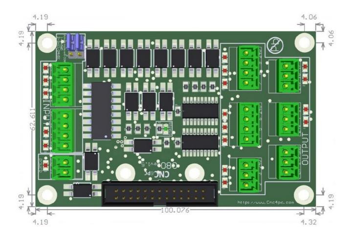
All dimensions are in Millimeters. Fixing holes (4mm).
