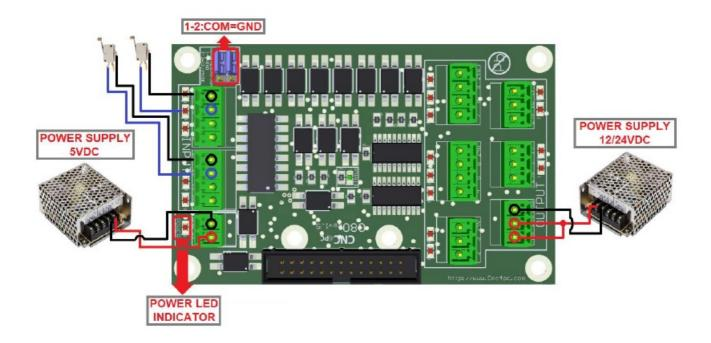
Wiring diagram to connect switches
