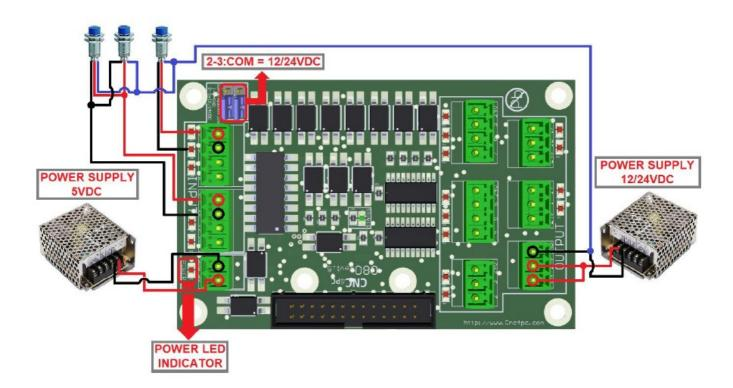
Wiring diagram to connect PNP open collector proximity sensors.
