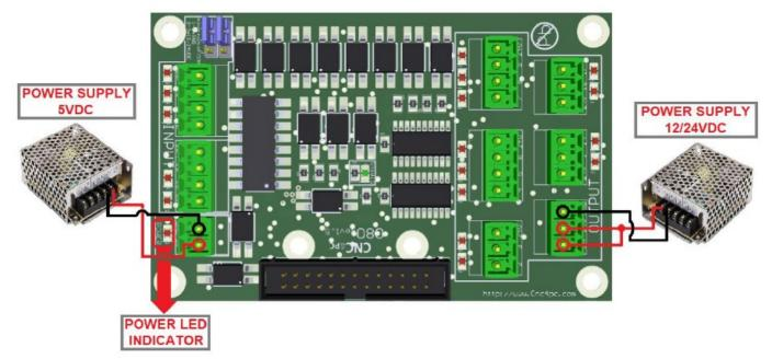
To preserve optoisolation two independent power sources should be used. A +5vdc to power the optos that interact with the controller (which could be a USB cable) and a +24vdc at 200mA to power the board.
