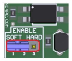
Use Hardware Enable to keep the driver enabled all the time. HARD ENABLE
