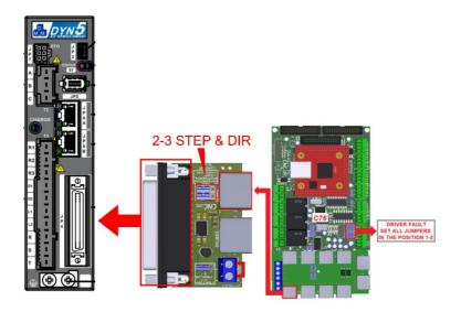
Diagram of connection with input signals Differentials, C74 and C76
