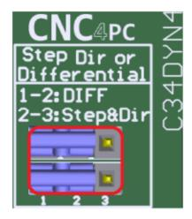
If not use the differential signal for STEP & DIR, set jumper as shown in the image
