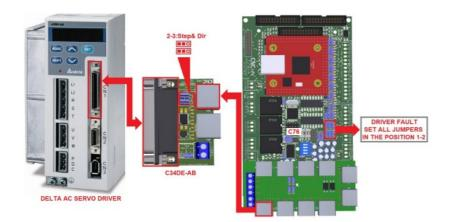
5.2 Diagram of connection with input signals Differentials C74 and C76
