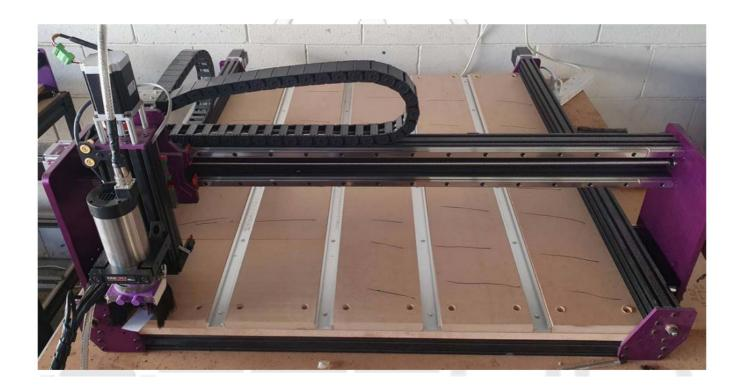
Using the jogging buttons in Commander, put a piece of scrap paper under the surfacing bit and lower the Z down until it is just touching the paper. Ensure to reduce your downward travel distance as you get closer to the surface to ensure the machine does not crash into the spoil board.
