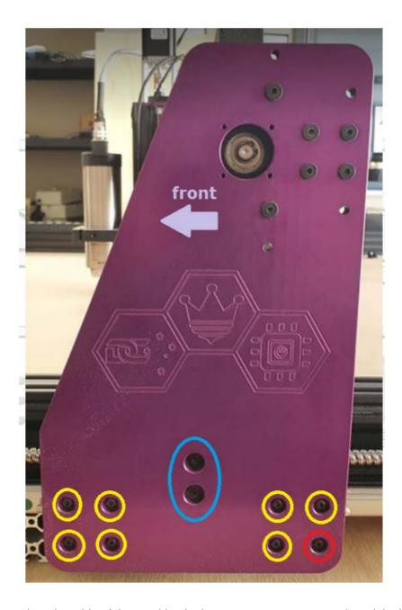
Repeat this process on the other side of the machine in the exact same pattern as the original side. This will allow us to "swing" the gantry front to back. Make slight adjustments at a time to both sides and re-secure the RED bolt first, then the YELLOW, then finally the BLUE bolts. Check if it is trammed correctly by cutting into your test piece. Repeat these adjustments until the test piece seems to surface quite flat with no ridges showing up as it skims the surface.
