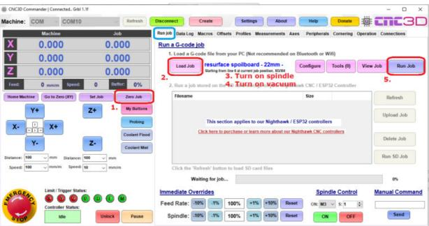
This will start the process of surfacing your spoil board. It may take a long time to complete this process. If something doesn't seem right then immediately hit the E- stop button on your control box or via our Commander software.
