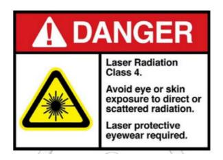
Always ensure you are wearing laser safety goggles and other appropriate PPE when using any high-powered lasers. Please ensure the laser is pointing away from people and sensitive materials.
