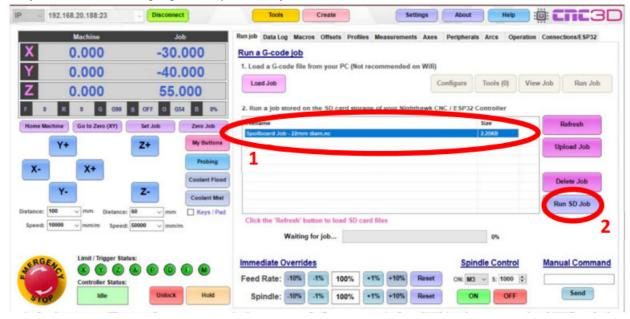
This will start the process of surfacing your spoil board. It may take a long time to complete this process. If something doesn't seem right then immediately hit the E- stop button on your control box or via our Commander software.
