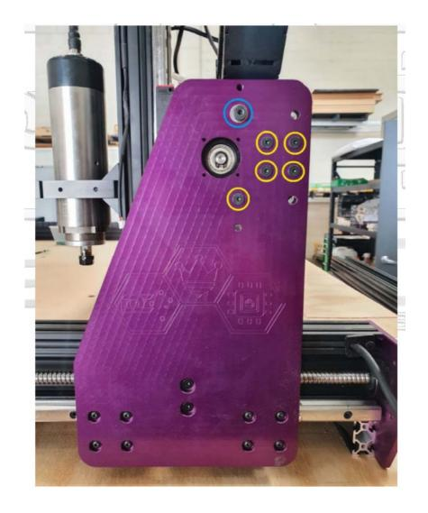
Repeat this process on the other side of the machine in the exact same pattern as the first side. This will allow us to "twist" the gantry front to back. Make slight adjustments at a time to both sides and re-secure the BLUE bolt first, then the YELLOW bolts. Check if it is trammed correctly by cutting into your test piece. Repeat these adjustments until the test piece seems to surface quite flat with no ridges showing up as it skims the surface.
