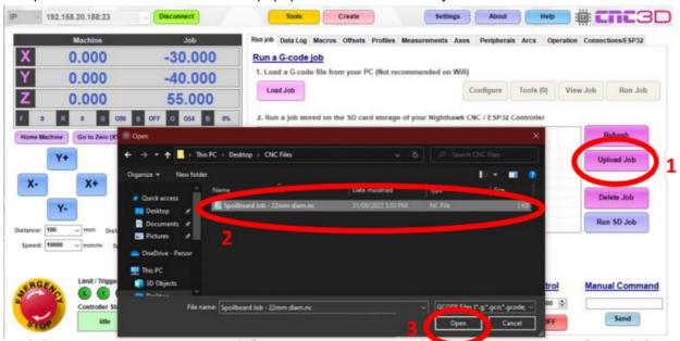
You're now ready to run the job! Attach your vacuum hose to the dust shoe turn on the extraction system, then turn on the spindle by pressing the Green button on the VFD. From there, all you need to do is highlight the spoilboard job in the list and click "Run SD Job"
